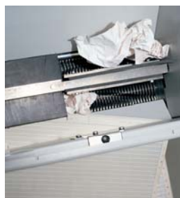
Automatic mechanical feeding system with revolving flaps
